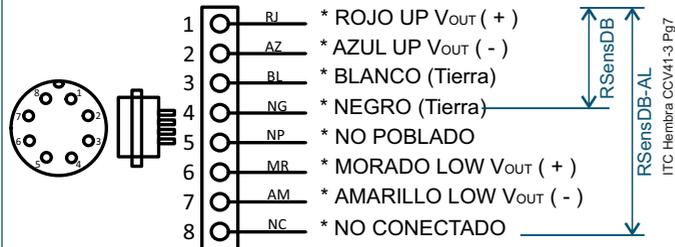
Conector cable-sensor RSensDB-S
